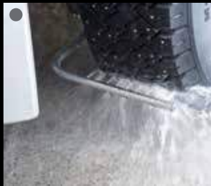
Dynamic steered wheel wash system
