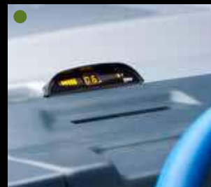
Acoustic distance warning system front
