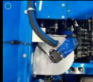
Washing system for vertical conveyor screw
