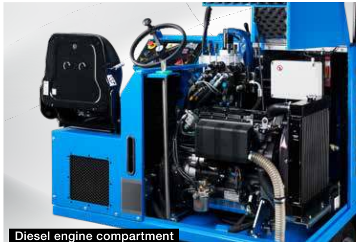
Diesel engine compartment
